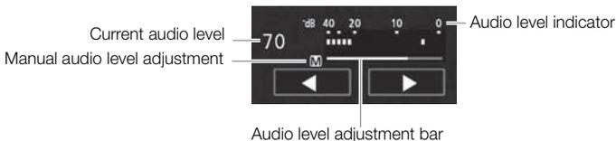
2 Touch and hold [◀] or [▶] to adjust the audio recording level as necessary.
