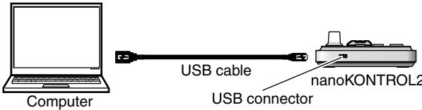
1. Use a USB cable to connect the nanoKONTROL2 to a USB port on your computer. The power to the nanoKONTROL2 will turn on and the power LED will light up.
